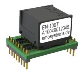
EMOSAFE EN-100T Network Isolators are intended for integration into printed circuit boards (PCBs) of electronic devices requiring advanced protection. The EN-100T can either be plugged into a socket or soldered directly to the circuit board. Due to their extremely compact design, they are still usable in very tight spaces. Additional TVS diodes protect individual wire pairs from voltage surges.
