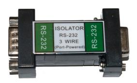
RS232 serial port isolator. DB9 female to DB9 male. The MI-RS912 isolator withstands 4000 VAC for one minute and supports speeds of up to 912600 bps. The MI-RS912 is one of the few RS-232 isolators on the market tested to EN60601-1-2. The compact isolator is powered by the serial port (10 mA maximum) and does not require any additional power supplies.
