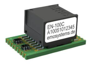
EMOSAFE EN-100C Network Isolators are intended for integration into printed circuit boards (PCBs) of electronic devices requiring advanced protection. The EN-100C is soldered directly to the circuit board. Their extremely compact design allows them to be utilised in situations where there is limited physical space. Additional TVS diodes protect individual wire pairs from voltage surges.
