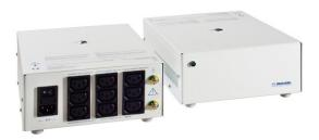
Isolation transformers, in a narrower sense, can also be called network transformers. The network voltage is transmitted lowloss to a secondary winding. This is isolated galvanically from the primary winding by means of a protective separation. The medical isolation transformers IMEDi and IMEDe increase the protection against electric shocks for patients and staff. Isolation transformers do not protect against electric shocks when one or both output terminals (Phase or Neutral) are touched.
