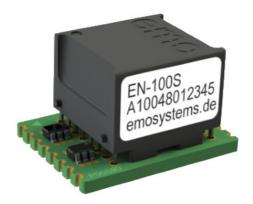
EMOSAFE EN-100S Network Isolators are intended for integration into printed circuit boards (PCBs) of electronic devices requiring advanced protection. The EN-100S is soldered directly to the PCB and features extra short solder terminals. Due to the extremely compact design, it can also be used in very tight spaces. Additional TVS diodes protect individual wire pairs from voltage surges.
