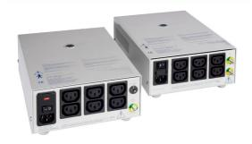
Isolation transformers, in a narrower sense, can also be called network transformers. The network voltage is transmitted lowloss to a secondary winding. This is isolated galvanically from the primary winding by means of a protective separation. The medical isolation transformers IMEDi and IMEDe increase the protection against electric shocks for patients and staff. Isolation transformers do not protect against electric shocks when one or both output terminals (Phase or Neutral) are touched.
