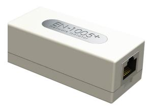
The EN-1005+ is equipped with transient voltage suppression (TVS) diode circuity. While conventional network isolators can only block voltage spikes that occur simultaneously at all signal lines (arising, for example, from potential voltage differences), potentially dangerous or damaging differential voltages on individual signal lines are clipped by the TVS circuity, preventing these voltages from reaching Ethernet devices, operators, and patients.
