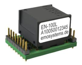
EMOSAFE EN-100L Network Isolators are intended for integration into printed circuit boards (PCBs) of electronic devices requiring advanced protection. The EN-100L potentially reduces the total mounting height of the assembly by being mounted from underneath the host PCB, protruding through a corresponding recess. Due to their extremely compact design, they are still in very tight spaces usable.
